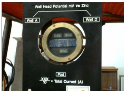
The ROV is interrogating the Sunstation monitor, mounted at the top of the SmartPod (pictured below).
