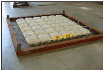
Concrete mattresses provide ample ballast to insure stability at the base
