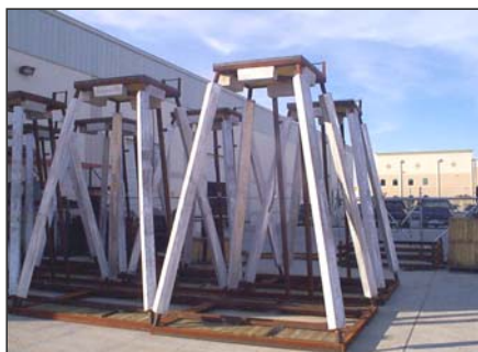
Concrete mattresses provide ample ballast to insure stability at the base
