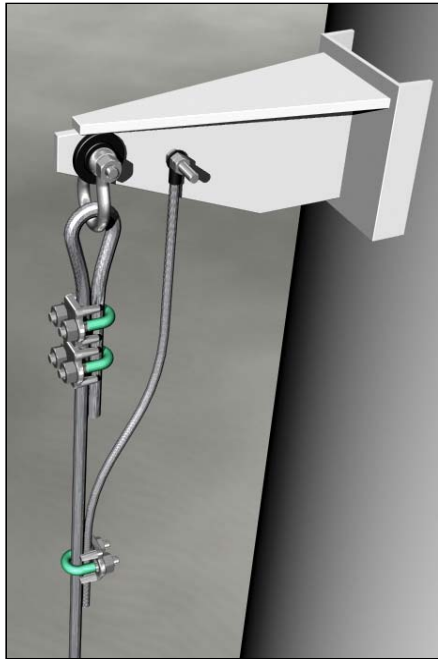
The weld-on standoff can be isolated for riser protection
