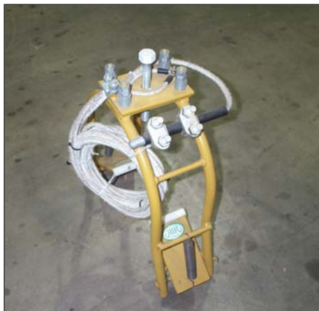
RetroClamp fitted with a V-String™ reference electrode.
