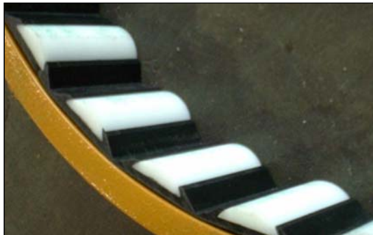
Up close: designed crevices in the composite construction channel water away from the pipe.
