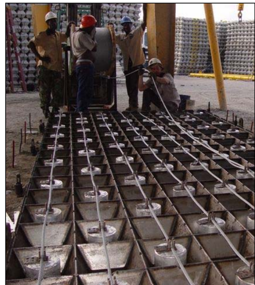
CP Mat shown in fabrication. Current and life requirements determine the number of anodes included.
